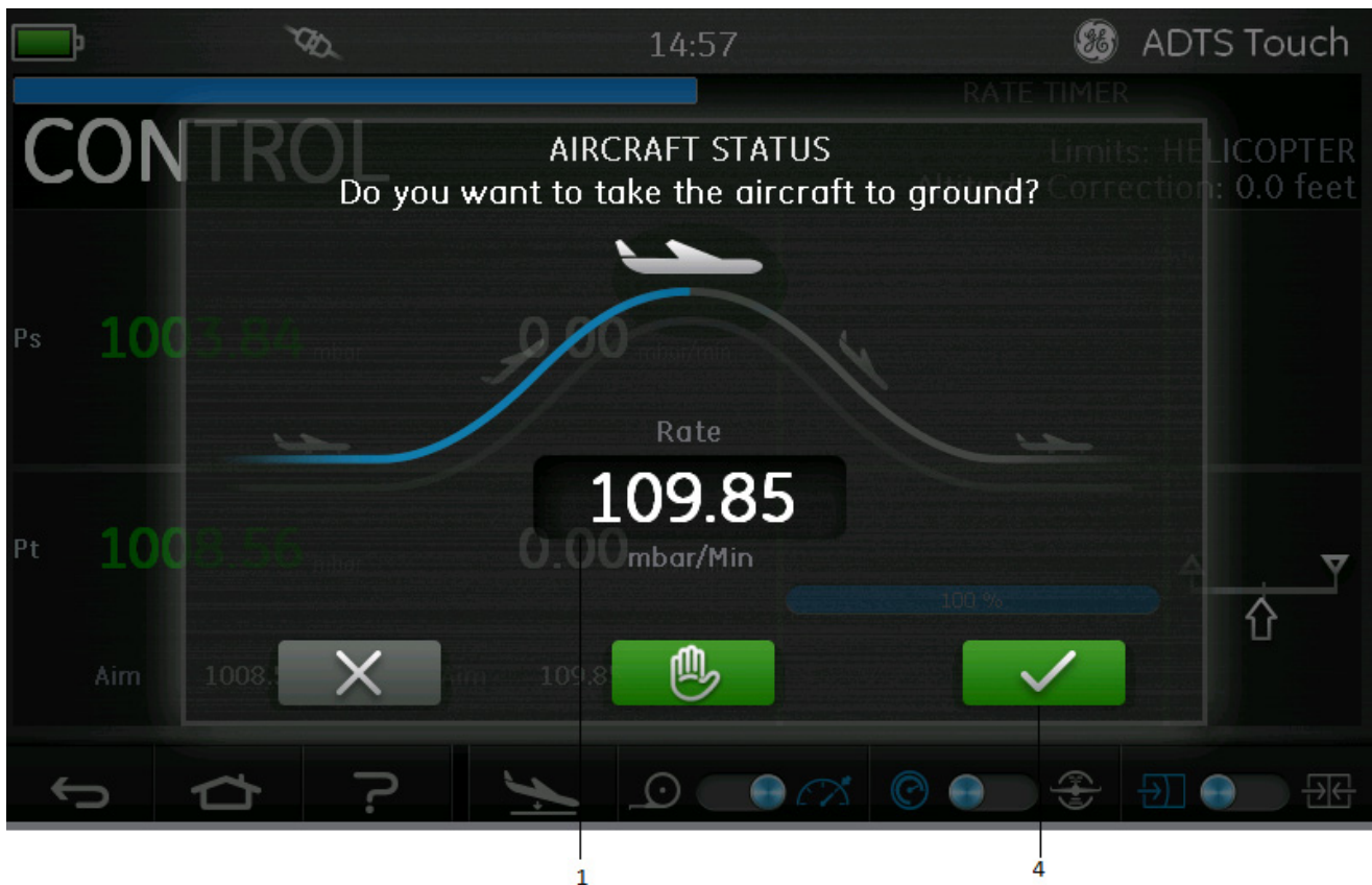
Figure 3-18: Go to ground main screen - Single Channel
