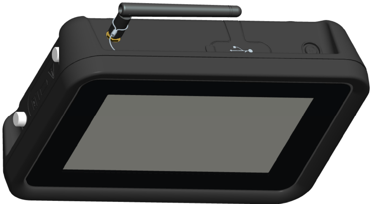
Figure 3-57: External Bluetooth® Antenna
