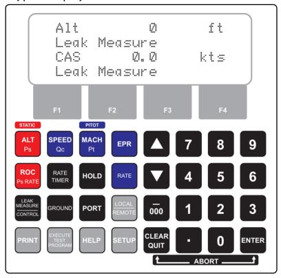
Figure 3-1: ADTS 405 Mk2 Keypad Display
