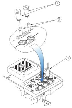
Figure 5-2: ADTS 405F Mk2 AC Fuse Positioning
