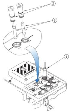
Figure 5-3: ADTS 405F Mk2 DC Fuse Positioning
