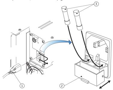
Figure 5-4: ADTS 405R Mk2 AC Fuse Positioning
