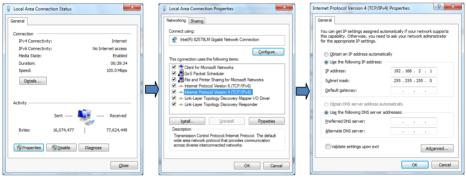
Figure 4-7: Configuring Windows For ADTS Subnet IP Address
